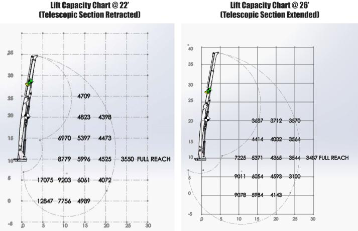
Note: The lift capacities shown above do not reflect the weight of a grapple or magnet. Grapple and/or magnet weights must be deducted from the above figures to gauge the lift capacity with these attachments.
