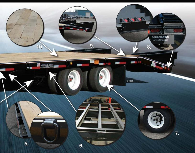
7.) Axles / Suspension - FT-10-2, FT-12-2 & FT-18-3: 6K Dexter Straight with Spring Suspension
