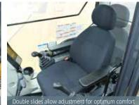
Operator seat can be adjusted independently of the control levers, and the entire operator seat assembly can be slid forward or back.
