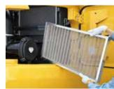
iNDr filter/radiator reservoir tank/air cleaner access.
