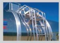
**Double Top Step Ladder** with Safety Handrails
