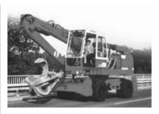
First hydraulic cab elevation
