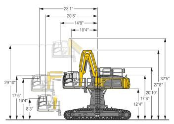
LHC-D 730 The hydraulically adjustable cab allows the driver, that he can choose his field of view freely and at any time within the stroke.
