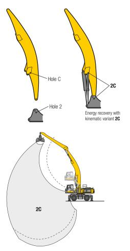
Altered range curve with additional reach depth, e.g. for unloading from ships
