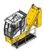
Hydraulic cab elevation
