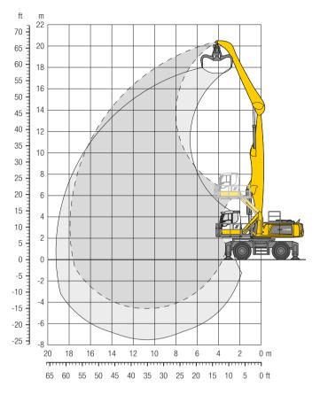
Height •• Can be slewed through 360° In longitudinal position of undercarriage
