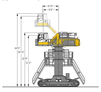
LHC 360-50 The hydraulically adjustable cab allows the driver, that he can choose his field of view freely and at
