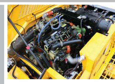
The layout of the engine, hydraulics and electrical, along with its forward-tilting hood and large side doors, make service and maintenance easy and accessible.
