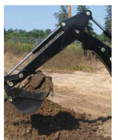
Several classes available depending on desired weight & digging force. 180° bucket rotation and swing arc. Heavy-duty construction grade available for heavy-duty applications. Equipped with cushioned cylinders.
