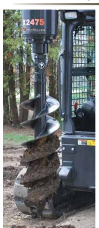
75 Series drive units are completely sealed with all moving components running in oil for total lubrication on a constant basis. The 75 Series hydraulic motor drives the auger through a sealed planetary gear reduction.
