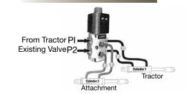
Used to convert existing tractor loader 2-function hydraulics to allow a 3rd function for controlling various hydraulic accessory attachments, for example hydraulic grapples and multipurpose buckets. Can plumb into existing loader bucket cylinder circuit.
