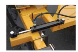
Angling capability powered by the tractor hydraulics
