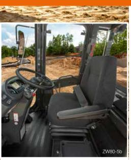
A standard long-stroke suspension seat absorbs shock and vibration (ZW80-5b).
