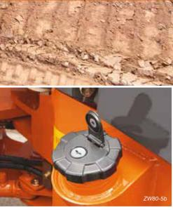
The fuel cap and engine cover can be locked with the ignition key.
