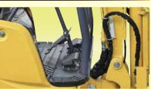
Pass-through operating station allows getting on and off from either side.
