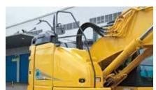
The handrail on the step side allows easy access to the maintenance port on the upper arm
