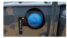
Urea filler cap is placed on the step for easy access.
