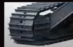
3 Heavy duty shoe (700 mm double bar grouser)
