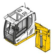
Hydraulic cab elevation
