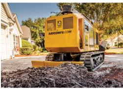
The wide hydraulic backfill blade saves time during clean up and can easily be folded in for passing through gates.
