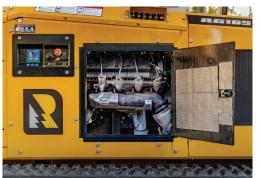
165 hp Ford gasoline engine provides cutting power without the hassle of complex, diesel after-treatment systems.
