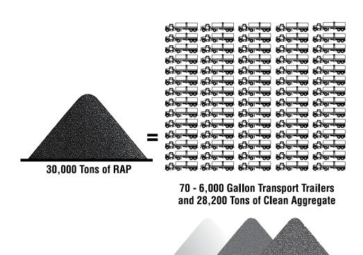
A 30,000 ton pile of RAP with an average 6% liquid AC content is the equivalent of about 28,200 tons of clean aggregate plus 420,000 gallons of liquid asphalt! This material can replace virgin materials in new mix. The recycled materials are as good as virgin rock or AC.
