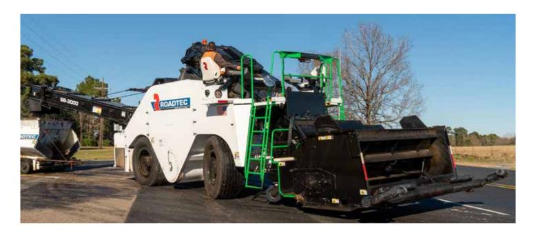
In the photo above, an intersection is being paved, however, the dump truck is not able to maneuver into the intersection. Therefore, the mix is deposited from the dump truck into the hopper of the SB-3000 and shuttled to the intersection where the mix is deposited into the waiting paver.
