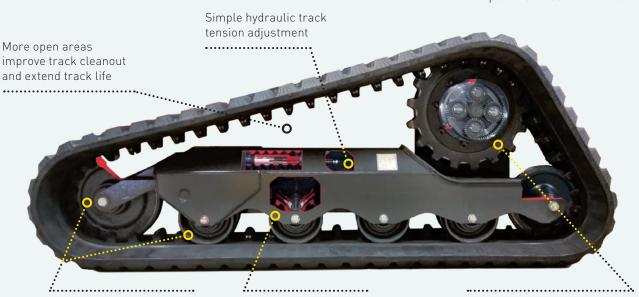
Lifetime sealed and lubricated rollers/idlers reduce maintenance costs Dozer-style triple flange rollers maintain tracking on inclines
