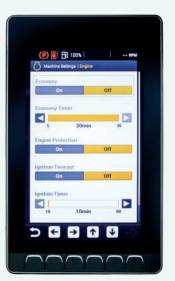
HAWK provides key operation data, including engine and performance information, RPM, fuel level, battery voltage, hydraulic oil temperature, engine temperature, and trip screen.
