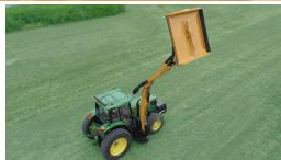
Maximum Reach of 30' Four bar linkage allows the cutting head to be maneuvered at greater angles making it easier to cut in hardto-reach areas.
