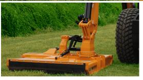
Mow Inches from the Tire 180° swing path allows the operator to mow within 6" of the tire.
