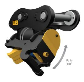
The D-Lock tilt has been designed with a compact narrow body for better visibility and performance, giving it serious benefits over other brands. The D-Lock Tilt allows operators to simply tilt all attachments rather than having to move the entire machine, improving the productivity and versatility of the machine resulting in increased profits. Mated with our rugged, triple-sealed power actuator, the D-Lock Tilt Coupler is built for virtually maintenance-free and trouble-free performance.
