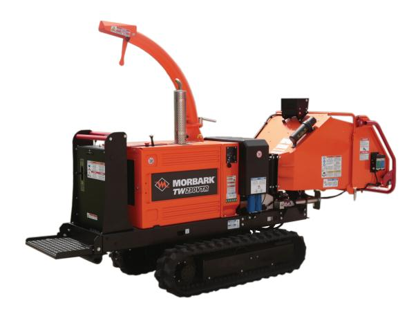
With a choice of a high-powered Briggs and Stratton Vanguard V twin gasoline engine or a high torque Kubota V1505 diesel engine, this wood chipper is a contractor's dream whether it's chipping or tracking to site. The TW 230VTR is ruthlessly efficient at getting the job done.
