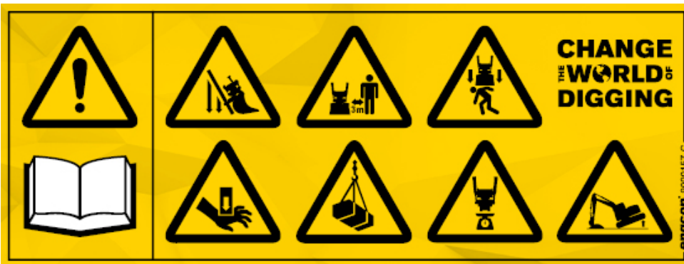
Figure 21. Warning decal to the right of operator.
