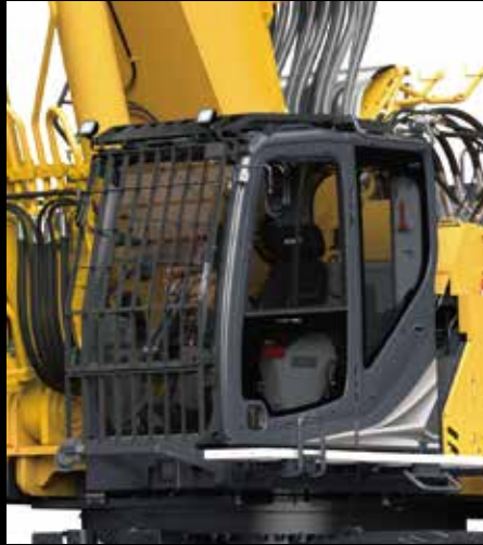
Front guard and Top guard are standard
