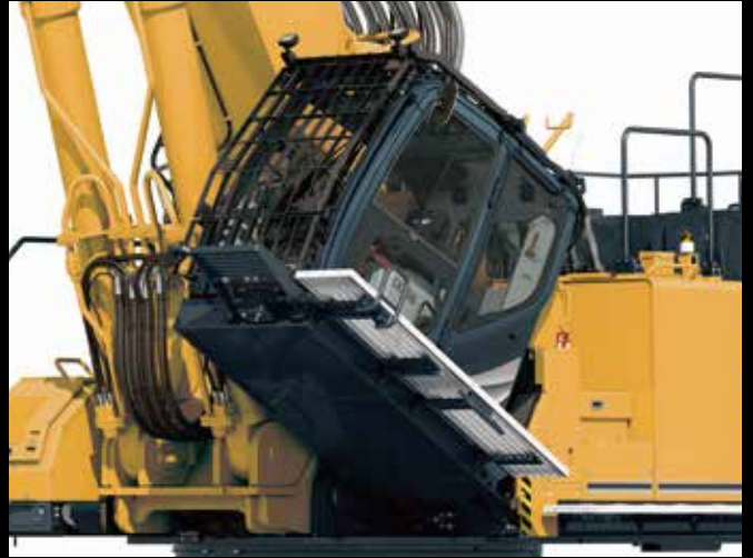
Cab can be tilted up to 30 degrees
