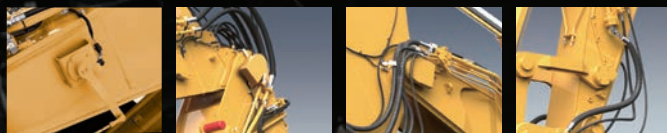
Boom angle sensor Jib angle sensor Arm angle sensor Bucket angle sensor
