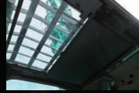
Vertical open/close roller shades to block direct sunlight.
