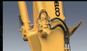
Safety valve for boom & arm & jib cylinder Prevents attachment from falling if piping is ruptured.
