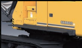
Catwalk Catwalks are installed on both the left and right sides at the base of the machine, providing easier access for maintenance.
