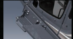
Cab entry step Positioned for convenient access to the tilt cab.
