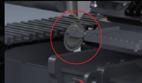
Cab lower mirror Check safety at foot areas and under the cab when tilted.
