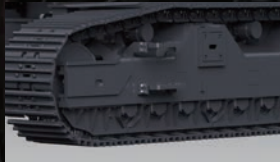
Full Track guide Prevents treads from coming off when mounting on demolition rubble.
