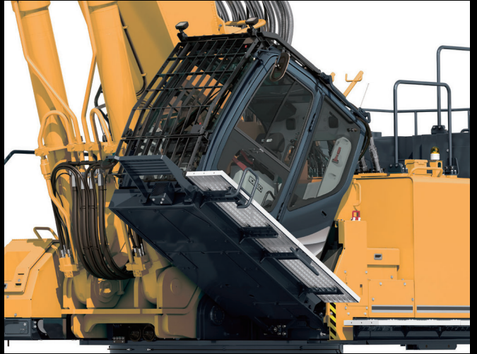
Cab can be tilted up to 30 degrees
