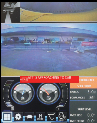
Cab interference warning display
