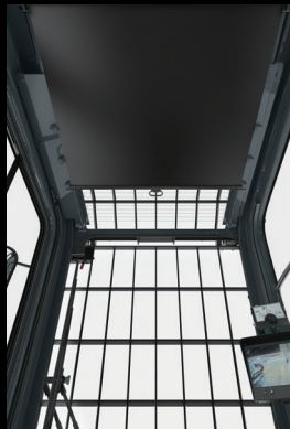
Sun screen for skylight
