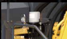
Auto lubrication system Quickly lubricate the attach- ments.
