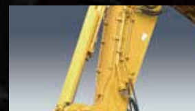
Bucket cylinder guard Prevents damage to the cylinder from falling debris.
