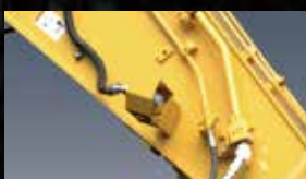
Water spray Drain circuit is provided for rust prevention.
