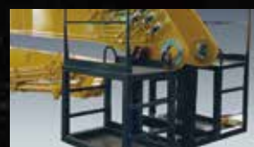
Attachment stand By standing on the side step, you can more accurately check the positions of the upper pin and connection hook during attachment assembly.
